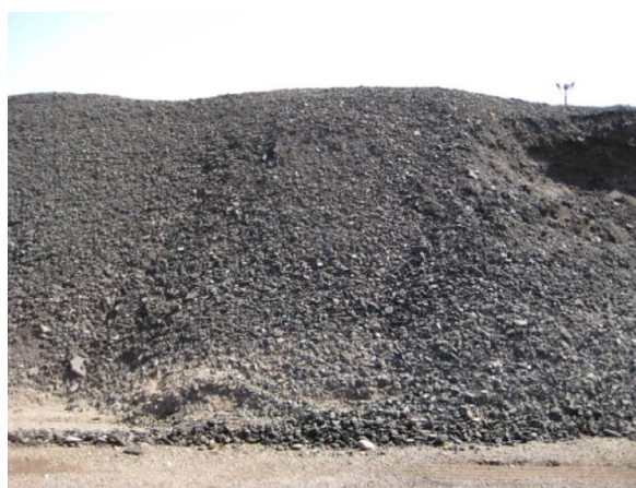
Stockpile of unprocessed RAP millings
